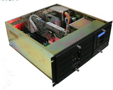
Reliable replacement computer for industrial clients who must have true ISA bus and PCI for their data acquistion and control add-on cards. Based on the last Intel 865G chipset that fully supports true timing of the ISA bus. Transduction has purchased enough 865G chipsets to support clients who need ISA slots for many years.
