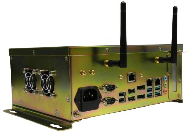
TR-ALDERLAKE-12 computer has been designed to offer high performance in a smaller chassis. The design is based on the 12th generation Intel i7-12800HE mobile processor with 14 Cores and 20 Threads. Operating range of temperature is  $0-60^{\circ}$ C ( $32-140^{\circ}$ F), it can be used as desktop or panel mount with included mounting brackets.
