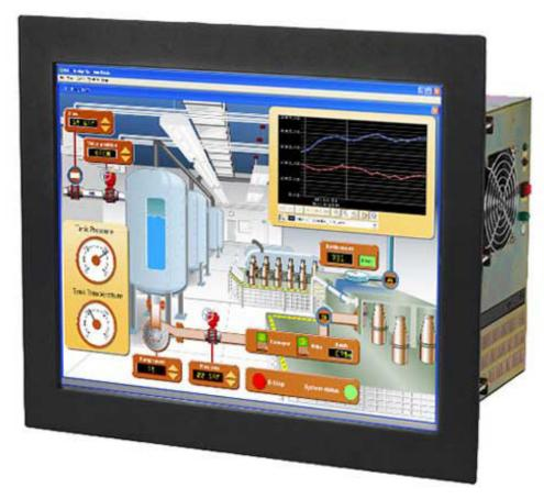
The TR-ALASKA is an all-in-one industrial panel or rack mount computer with extended temperature range down to -20°C (-4°F). It can be supplied with modern multicore i5/i7 Intel processor or in legacy version for compatibility with older Microsoft operating systems. Optional power is 120VAC, 220VAC or 24VDC, 48VDC, 125VDC and 250VDC.
