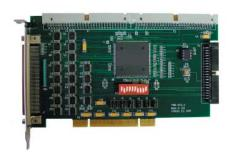
QP option modules are plug-and-play replacements for popular legacy Digital interfaces. Option modules install in a PDQ-3200 system and offer the same functionality as the Digital equivalent, thus allowing users to migrate from their Qbus systems to 3200 systems and maintain their investment in software and user equipment.
